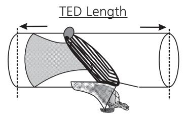
If webbing immediately around TED has a mesh size smaller than allowed for the trawl, such webbing may not be greater than 60 total stretched meshes in length.
